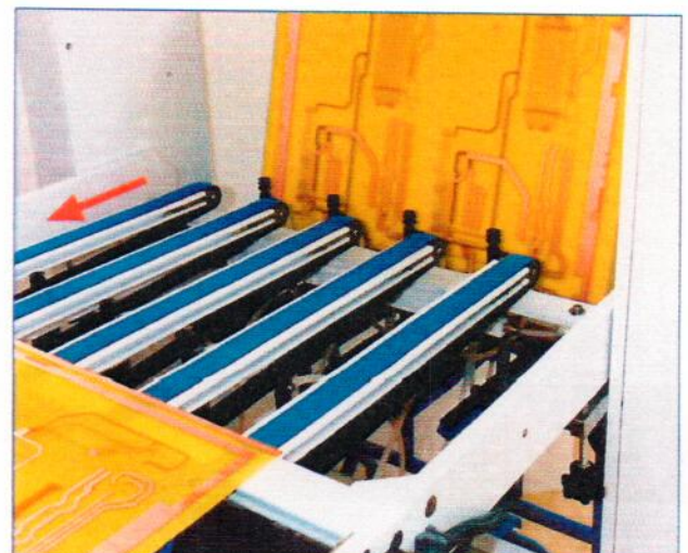
• PCB board exits the Jiraf conveyor.
