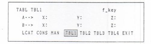
This is the first level of the table operation tree. There are three table moving operations, LCAT (location movement), CONS (constant distance movement), and MAN (manual movement). Select the required operation by pressing function keys 1, 2, or 3. Then use function keys 4 to 7 to specify which table is to be moved.
