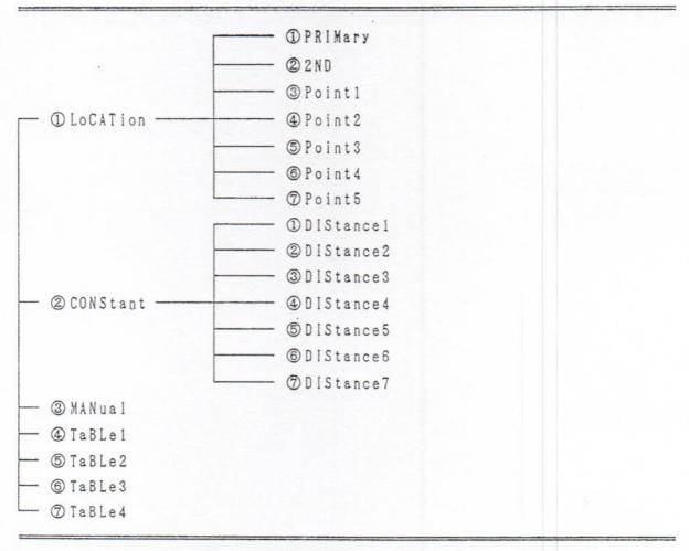
Press the TABLE switch of the OPERATION group twice to produce the following function key display at the bottom of the CRT screen.
