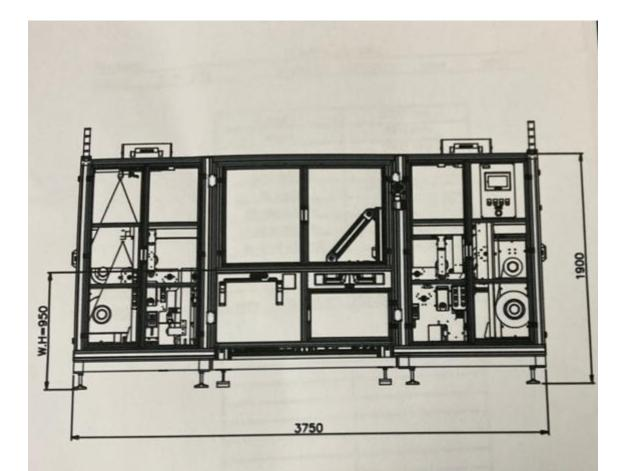
The production line consists of three modules, at the beginning an unloading, at the center the AOI control system, and finally the loading.
