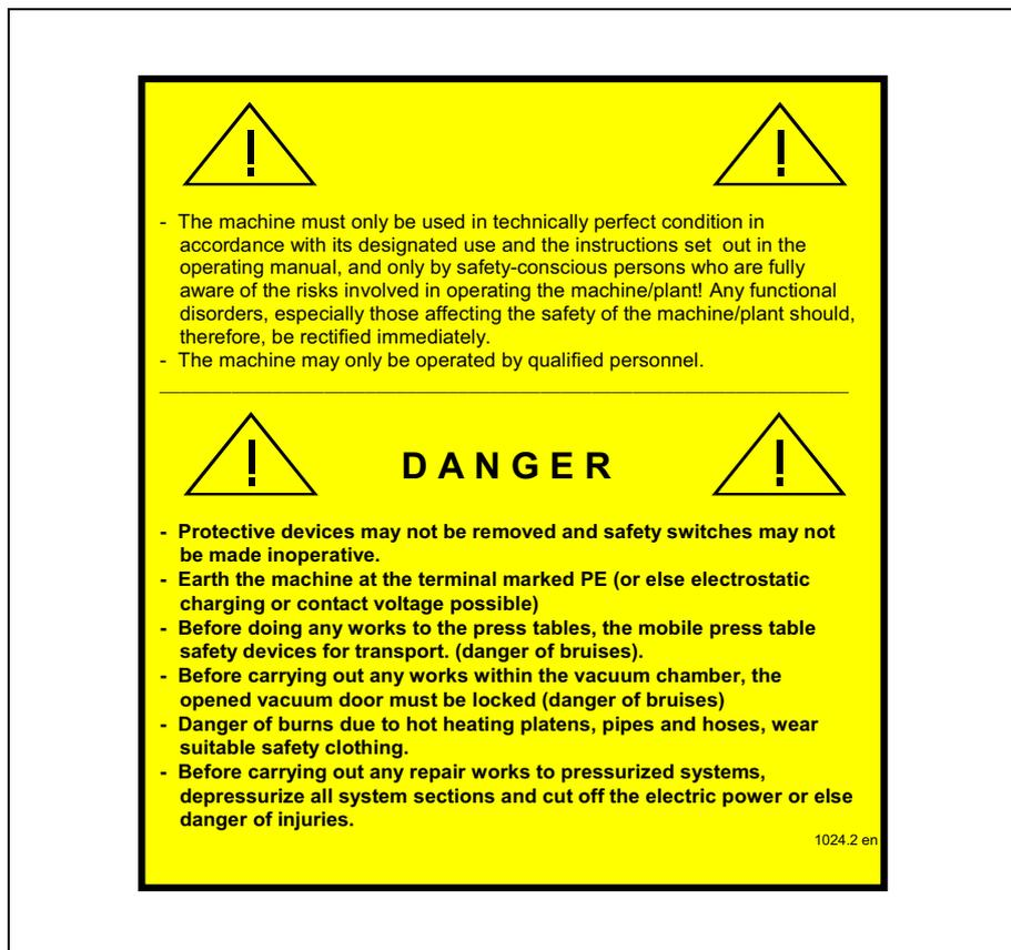
**Figure 2-4** Warning sign 3 (on the switch cabinet)
