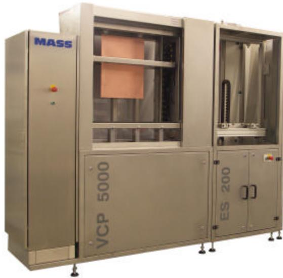
This machine is designed to fill holes in printed circuit boards with conductive or non conductive paste. The hole filling can be performed with through-hole vias and blind vias. The filling of blind holes is possible in a double side mode in one step. The machine is equipped with a glass cover for visual quality control on both panel sides.
