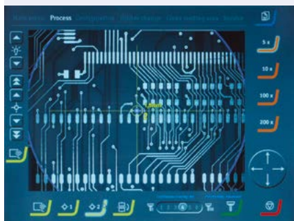
Vias to be inspected are first pointed out at low magnification (5 or 10 x). Here shown in 5 x mag.
