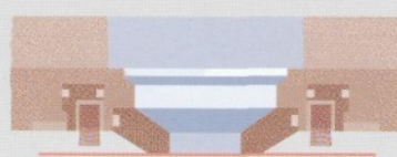
Stegfreies Fräsen m/t Druckring Pinless routing with pressure ring
